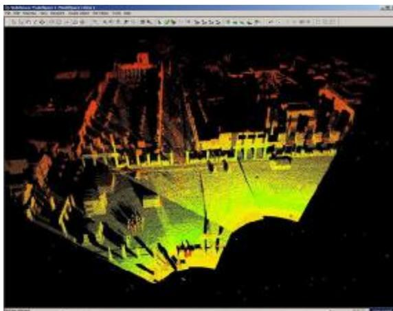
Fig. 8: Image in untrue colours of part of the 3D model, obtained by the superimposition of three scans.
