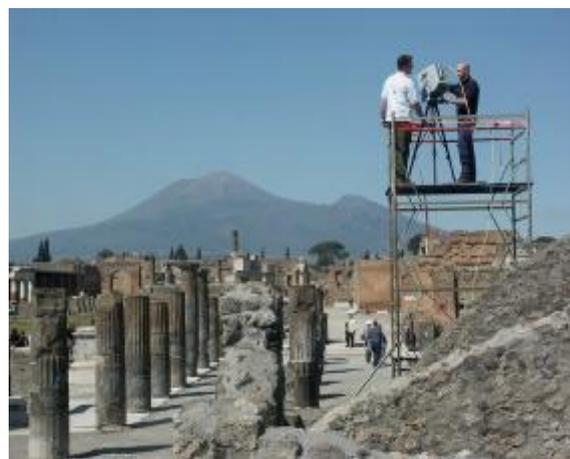
Fig. 3: The Forum of Pompeii during the 3D surveying process: in foreground the laser scanner Cyrax 2500
