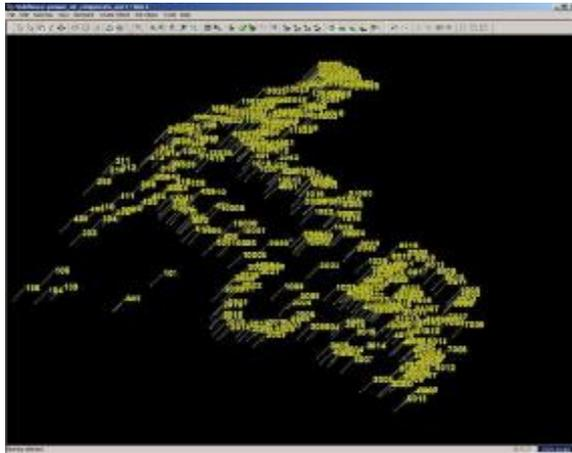
Fig. 6: Cloud of points surveyed by the TCR 1101 total station, imported in "Cyclone"© software to insert the scans in spatial co-ordinates
