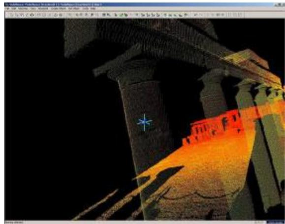
Fig. 4: "Cyclone"© software acquiring automatically a tie point (target).
